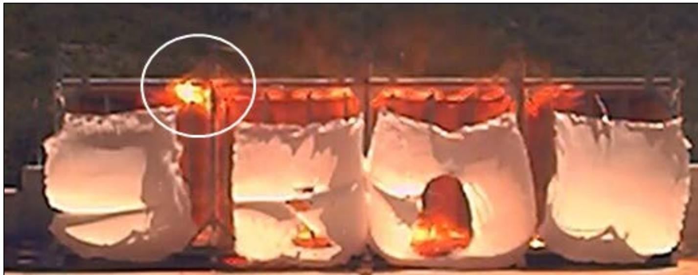
**Figure 11. Test B02 – HS Video – Left Side DDT Location (0.66 ms after Figure 10)**
