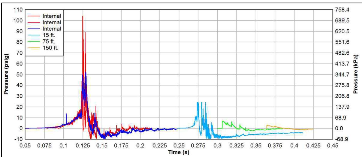
**Figure 9. Test B02 – Pressure-Time History for Select Gauges**
