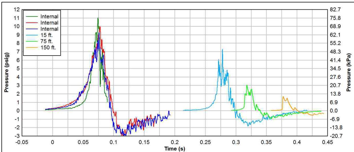
**Figure 6. Test B01 - Pressure-Time History for Select Gauges**
