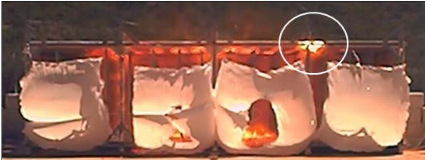
**Figure 10. Test B02 – HS Video – Right Side DDT Location**
