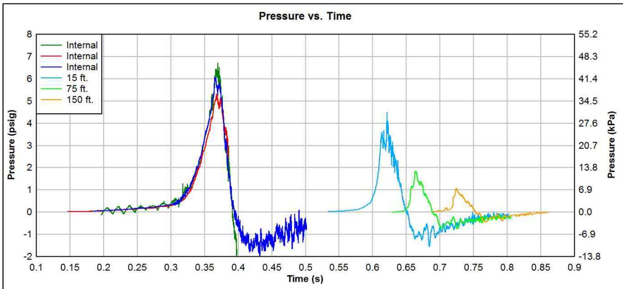
**Figure 4. Test A02 – Pressure-Time History for Select Gauges**
