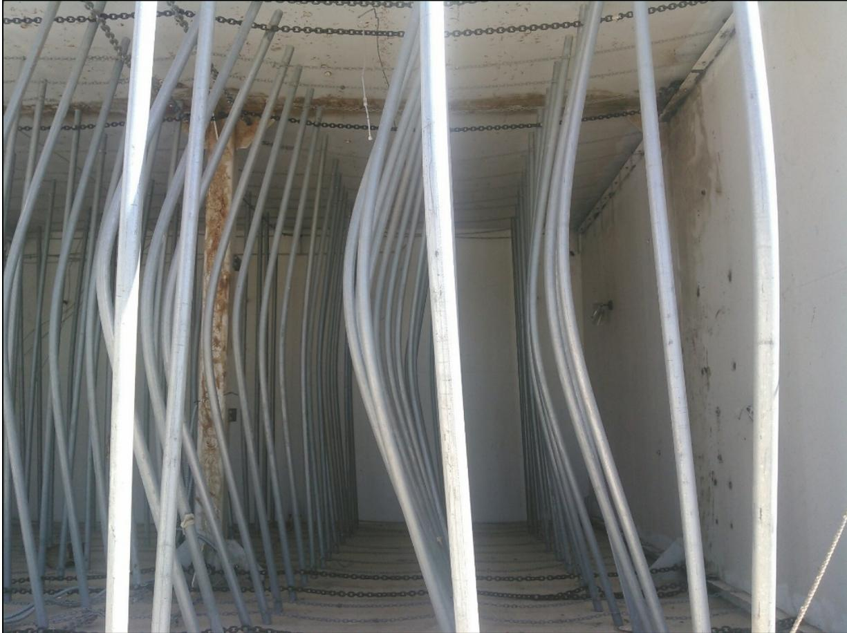
**Figure 13. Photo of Pipe Deformation following Test B02 DDT**
