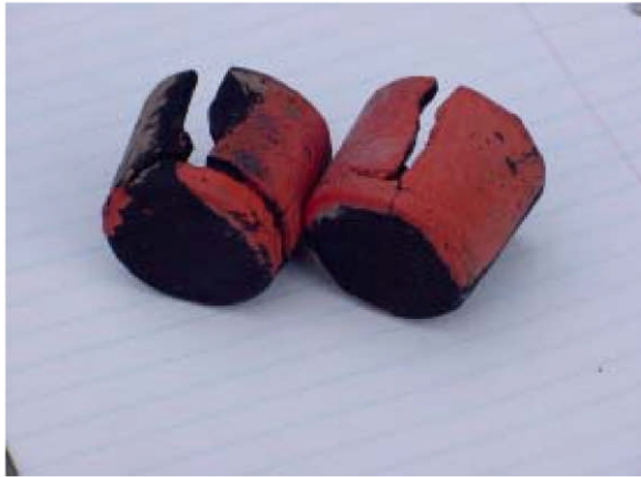
Figure 4. Two vent caps, typical of the four vent caps found at the site.
